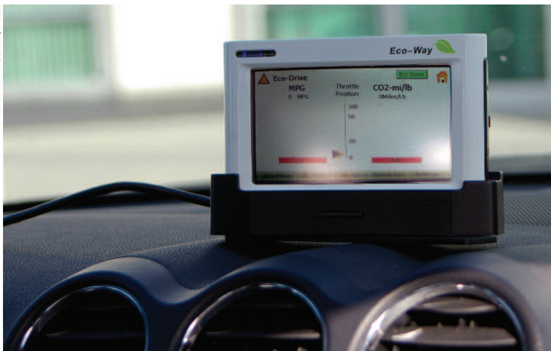
The Eco-Way device, deployed by researchers at the University of California, Riverside, allows drivers to monitor fuel usage as they drive.
