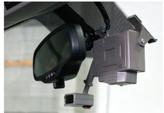
(Right:) A head unit, attached near the rear-view mirror, comprises cameras recording four different fields of view. It also receives data from accelerometers and a passive alcohol sensor.
