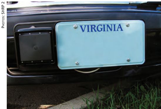
(Left:) A forward radar unit, mounted near the license plate, is among the data-gathering devices installed in participant vehicles.
