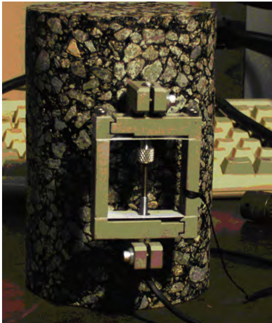
A mounted magnetic extensometer measures strains for the dynamic modulus test on a pavement specimen. The development of a simple performance tester for routine hot-mix asphalt design is one of many NCHRP projects that have advanced the practice of pavement design.
