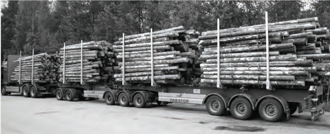
A 30.5-m, 90-ton timber truck, called “en trave till,” undergoes testing in Sweden for hauling timber on specified routes. Longer and heavier truck combinations for transporting timber and mining products are a challenge for low-volume roads in the Nordic countries. ROADEX research has identified axle and tire configurations and tire pressures to make the trucks more road-friendly than standard trucks and to reduce haulage costs and carbon dioxide emissions per haulage ton.
