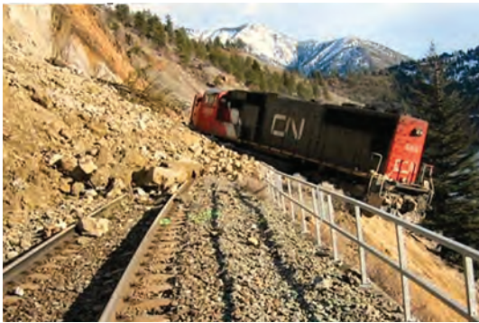
Small rockfall debris pile on tracks near Lytton, British Columbia, caused a train derailment in January 2007.
