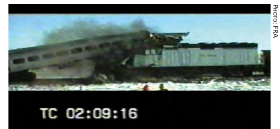
A frame from the conventional train-to-train impact test captures the moment of override.
