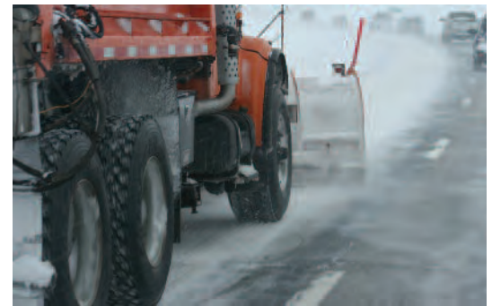
Winter operations contribute to the rapid deterioration of markings.
