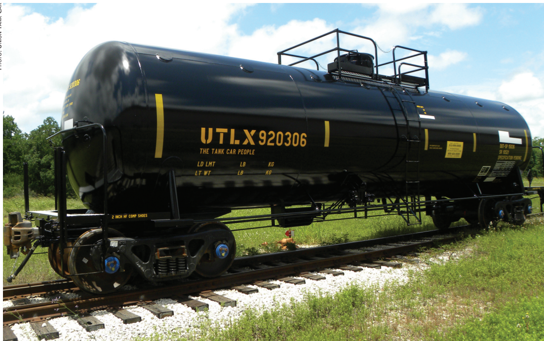
Design of the new DOT-117 tank car, one of the "Tank Cars of Tomorrow," applied findings from the Next-Generation Rail Tank Car Program.
