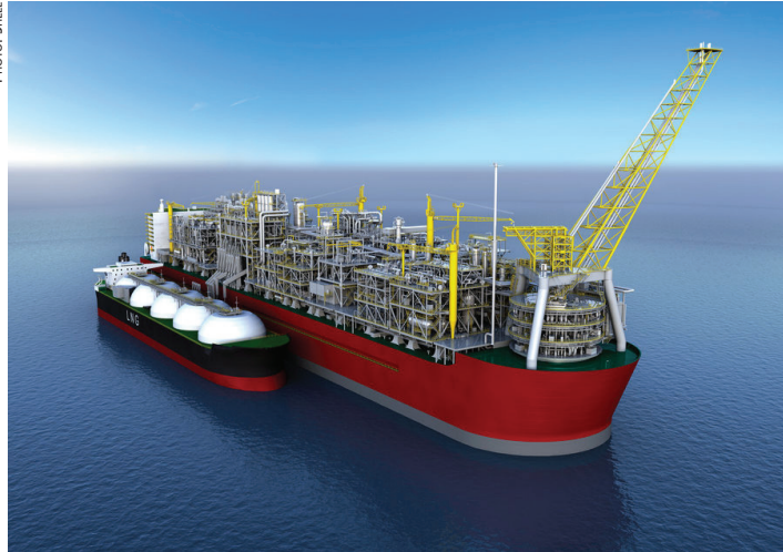
Shell's floating LNG facility Prelude can transport LNG directly to carriers at sea.
