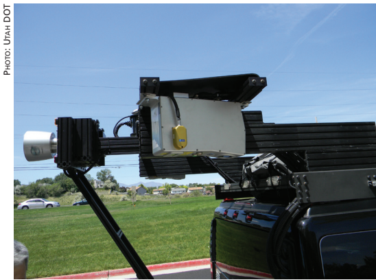
Equipped with a lidar camera, this Utah DOT data-collection vehicle collects high-definition, 3-D representations of surrounding areas.
