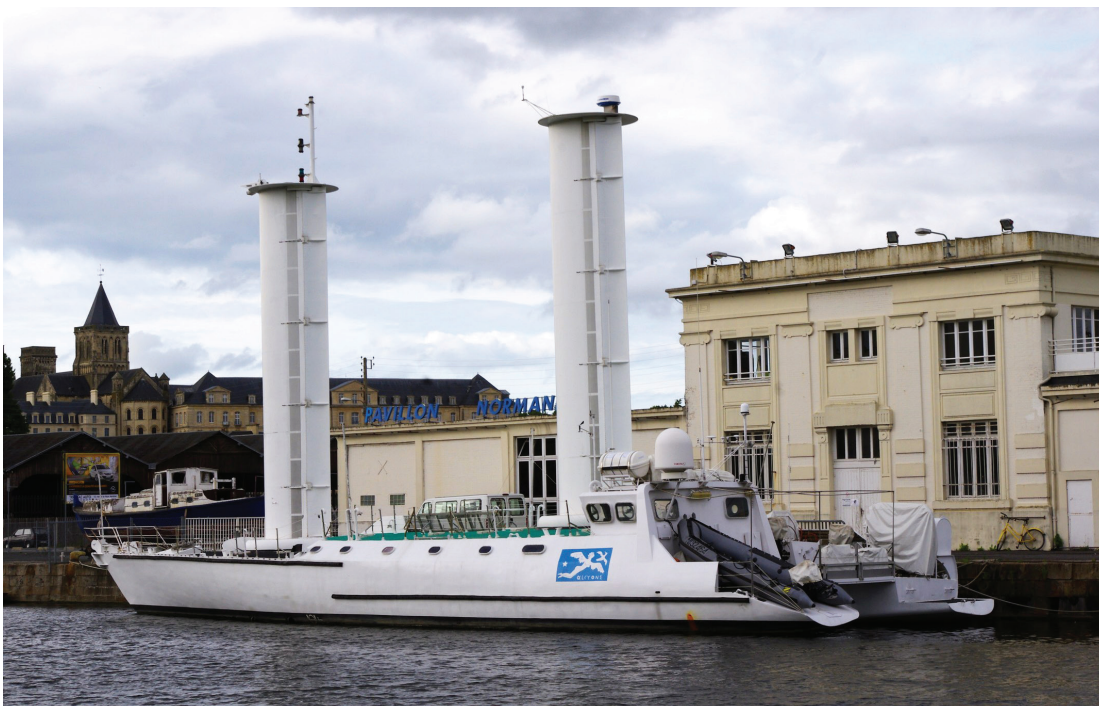
Flettner rotors, like those on the ship Alcyone , augment traditional engines to generate electricity.
