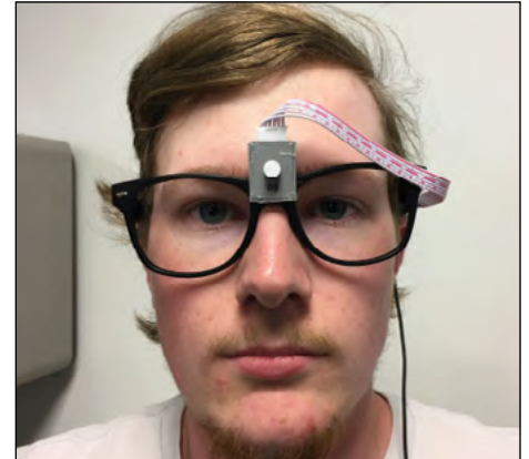
FIGURE 1 Personal light dosimeter developed at Virginia Tech Transportation Institute.
