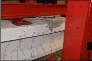
Concrete crushing Compression failure
