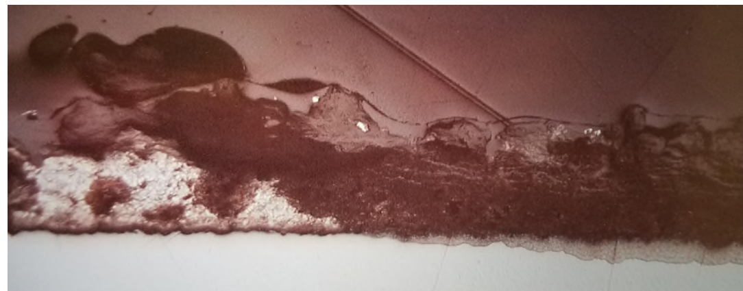
Image taken using Optical Microscope after 5-yrs. in the salt fog chamber (350x).
