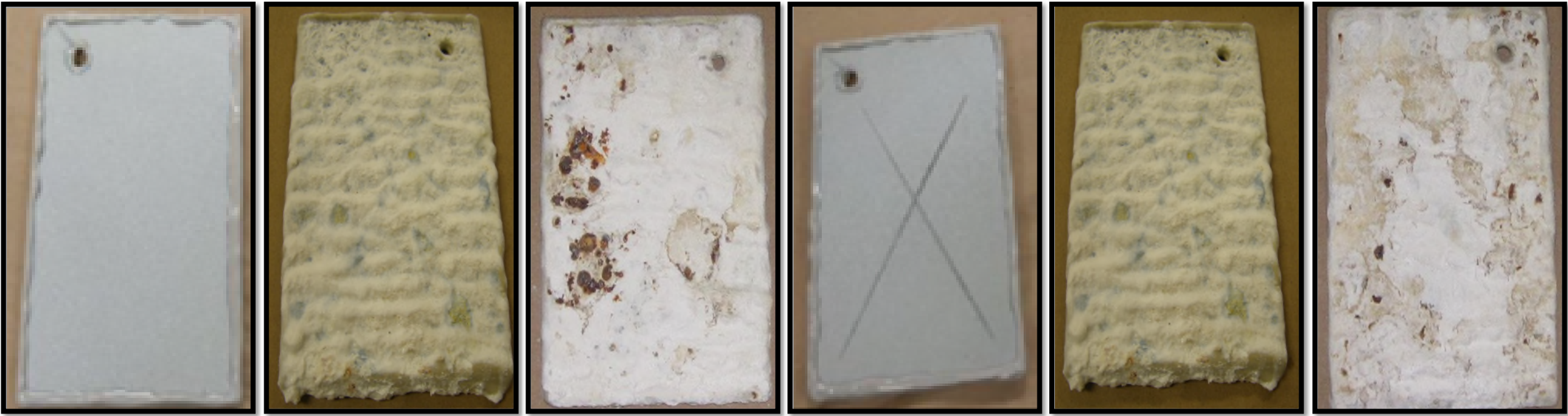
Condition of the panels at 0 hrs., 30,000 hrs., 5 years; Left (Unscribed) & Right (Scribed)
