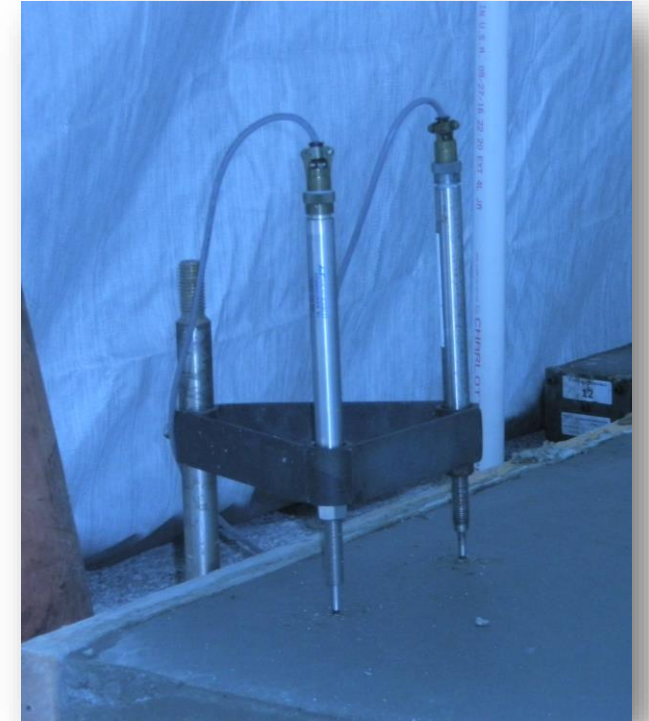
Linear Variable Differential Transformer (LVDT) measurement of slab corner lift-off
