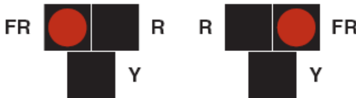
5. Alternating Flashing Red During Pedestrian Clearance Interval
