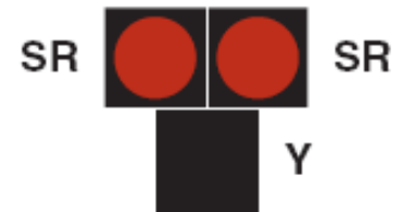
4. Steady Red During Pedestrian Walk Interval
